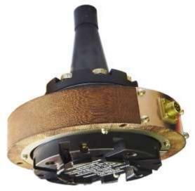
The M44 measures 4 components of force (Fx, Fy, Fz) along the three orthogonal axis (X, Y, Z) and torque (Mz) during the rotating. The M44 can be used for logging of the friction stir weldind (FSW) parameters.
